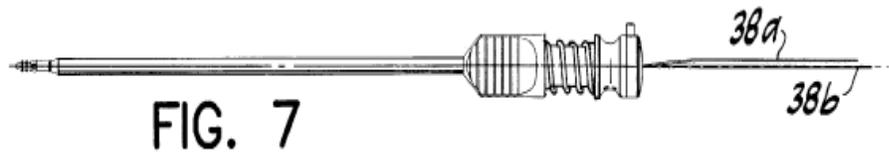
Figures 1 and 7 depict a suture anchor driver according to Fucci's invention. As shown in Figure 1, driver 10 includes drive shaft 12 extending to distal end 16, and handle portion 18 at proximal end 20. *Id.* at 4:26–30.
