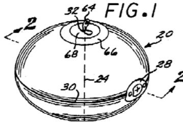
Gau’s gastric balloon also includes a self-sealing valve (element 28, Figure 2 reproduced below), a fill tube guide (element 54, Figure 2 reproduced below), and a removal tab (element 64, Figure 2 reproduced below).
