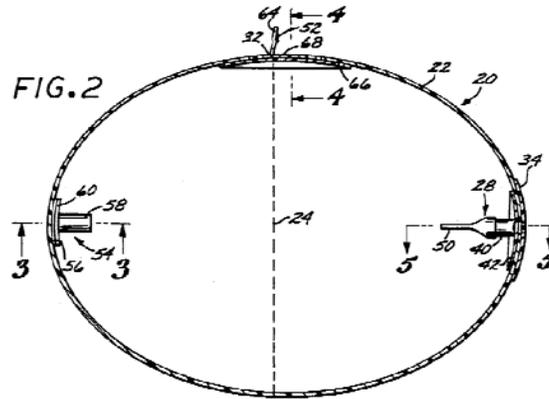
“The purpose of the valve 28 is to permit inflation of the balloon 20 after it has been inserted into the stomach 26, and also its deflation before it is desired to remove the balloon 20 from the stomach 26.” (Ex. 1008, Col. 4:56-60.) “The purpose of the fill tube guide 54 is to serve as a seat for the stiffening rod or stylette (not shown) which is used to make the fill tube and balloon rigid during the original insertion of the balloon 20 into the stomach 26.” (Ex. 1008, Col. 6:51-55.)
